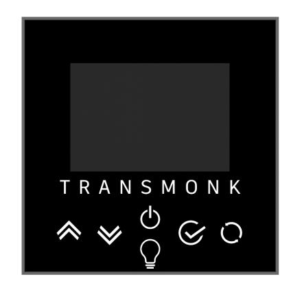
The controller is designed/programmed to switch over working between 2 pumps in a controlled way as per set points. It is equipped to set and varies the working time of each pump while working. In case of any fault in one pump it automatically switches the complete working to another and create alarm signal which help to avoid any damage due to uncertain issues in pumps. The display is user friendly and keep on updating about health condition of both the pumps.
